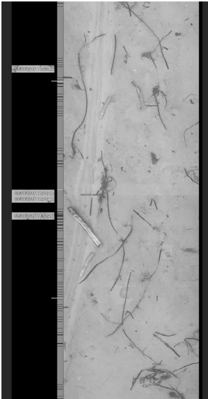
Figure 19: Part of the vertically stitched video for Trip 1, Tow 1. Stitching appeared generally good with problems in pattern matching only occurring where multiple objects moved between frames. The grey blocks down the left edge of the track indicate stitched frames, the short white ticks indicate 0.5 m distance marks and the longer white ticks, 1 m distance marks.
