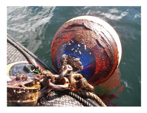
**Figure 6:** Light fouling of barnacles and mussels on mooring, with mussels visible on the mooring chain.
