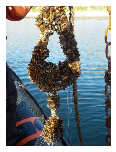
Figure 7: Heavy fouling of mussels on mooring rope.
