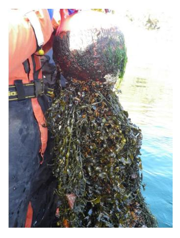
Figure 4: Typical fouling of algae and mussels on mooring
