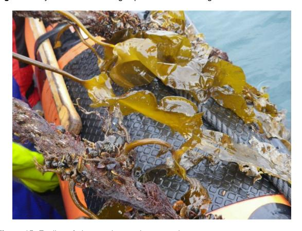
Figure 15: Fouling of algae and mussels on mooring ropes.
