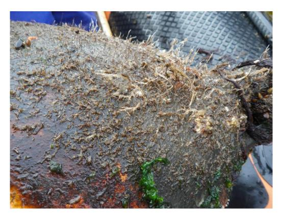
Figure 14: Hydroids and some algae present on a mooring.
