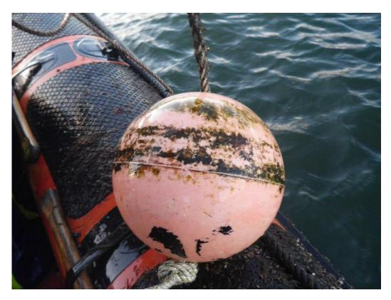
Figure 13: Light algal biofilm on mooring.
