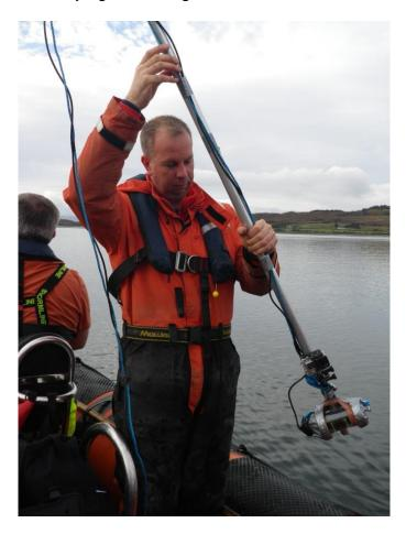
Figure 3: Pole-cam with GoPro attached.
