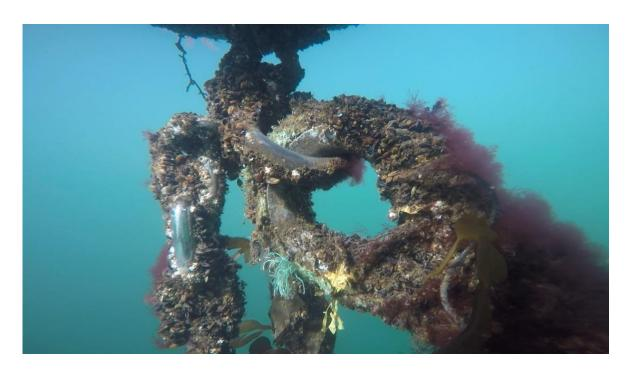
Figure 22: Video footage still of vessel mooring chain.
