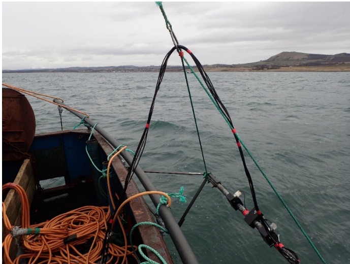
Figure 4: The video-rig being lowered off the back of the vessel from the fixed stern derrick, the grey bar resting on the gunwhale is the electrode spreader which was lowered once the video rig had settled on the seabed, the black video cables and orange electrofishing power cables can also be seen.
