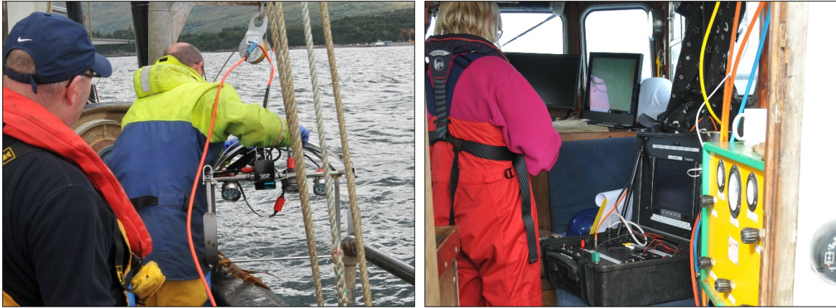
Figure 4: The NatureScot mini-DDV system used as a back-up on the first survey of the project, deployment from chartered vessel ( Lady Nicola ) and surface control unit in the wheelhouse (black peli-case on the seat).
