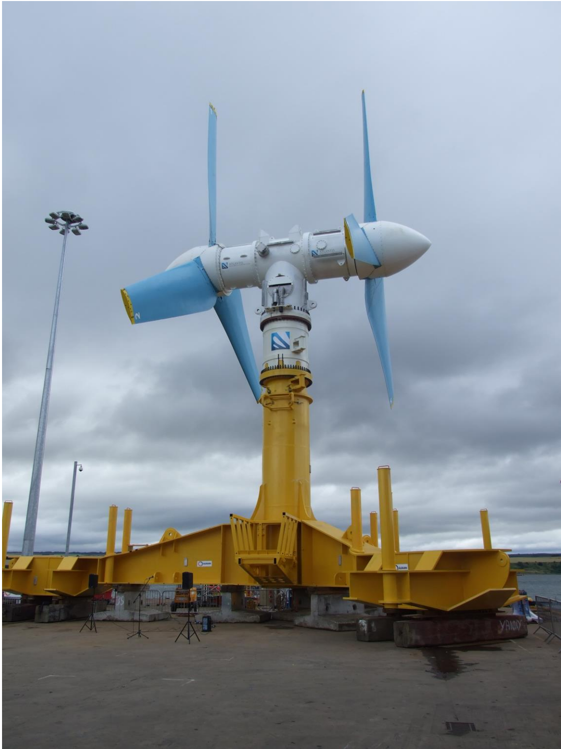
Figure 1: Atlantis Resources Corporation AK-1000 tidal current turbine set to be deployed for the MeyGen project at the Pentland Firth (EMEC, 2011).
