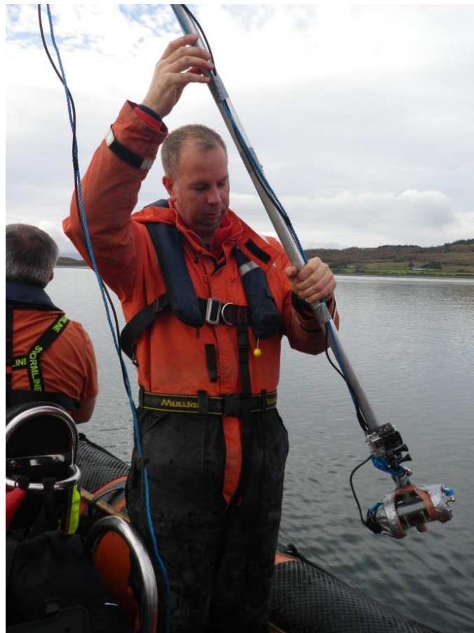
Figure 3: Pole-cam with GoPro attached.
