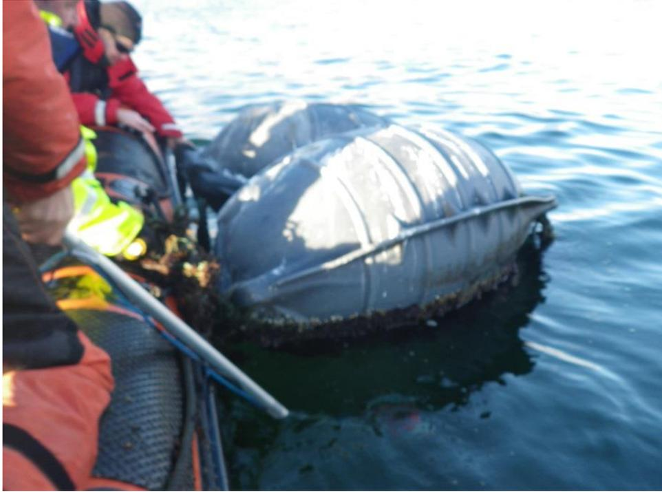
**Figure 2:** Pole-cam surveying a mooring.
