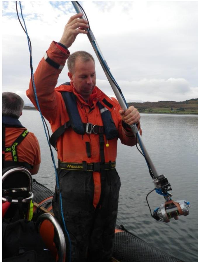
**Figure 3:** Pole-cam with GoPro attached.
