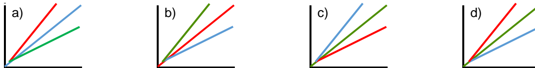
Figure 3: Earned value reporting graphics. Red = planned costs, blue = actual costs, green = earned value.
