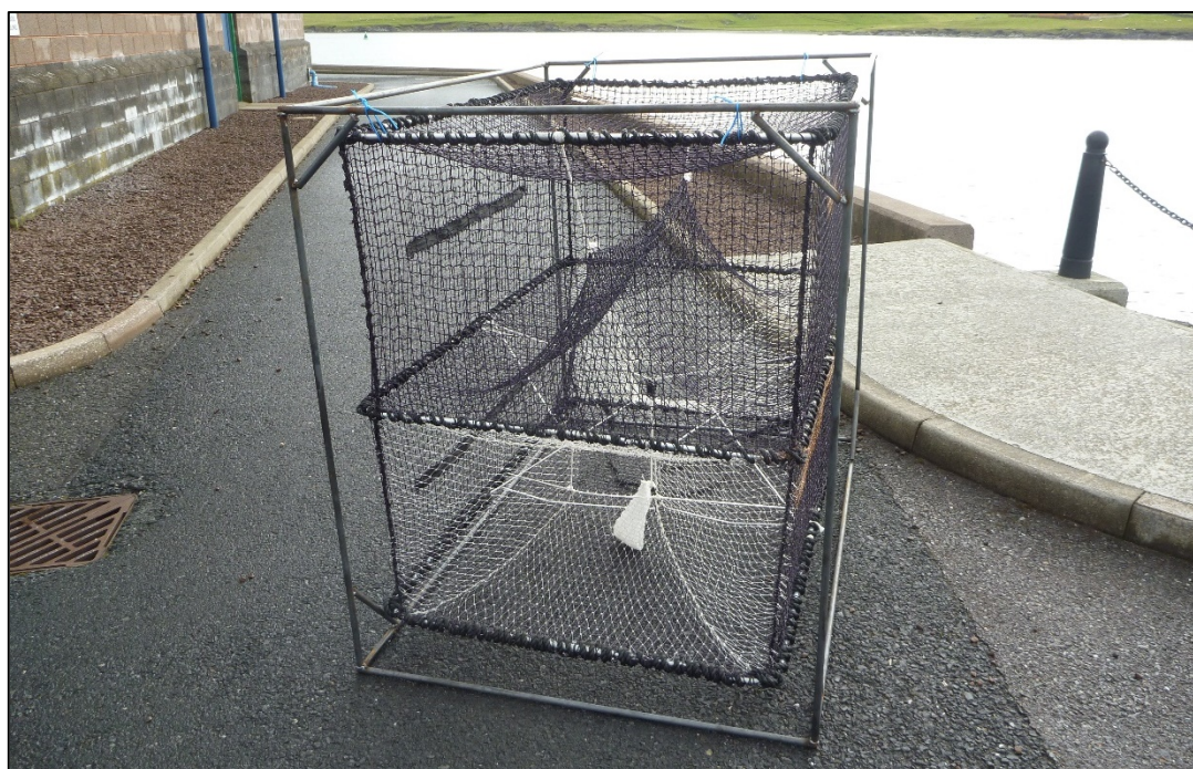
Figure 1: Carapax collapsible trap rigidified within a frame constructed from 16 mm rod iron. © NAFC
