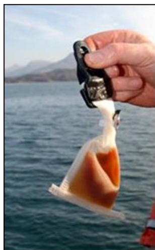
Figure 11.2 SPATT bag used by MSS for lipophilic toxins monitoring.
