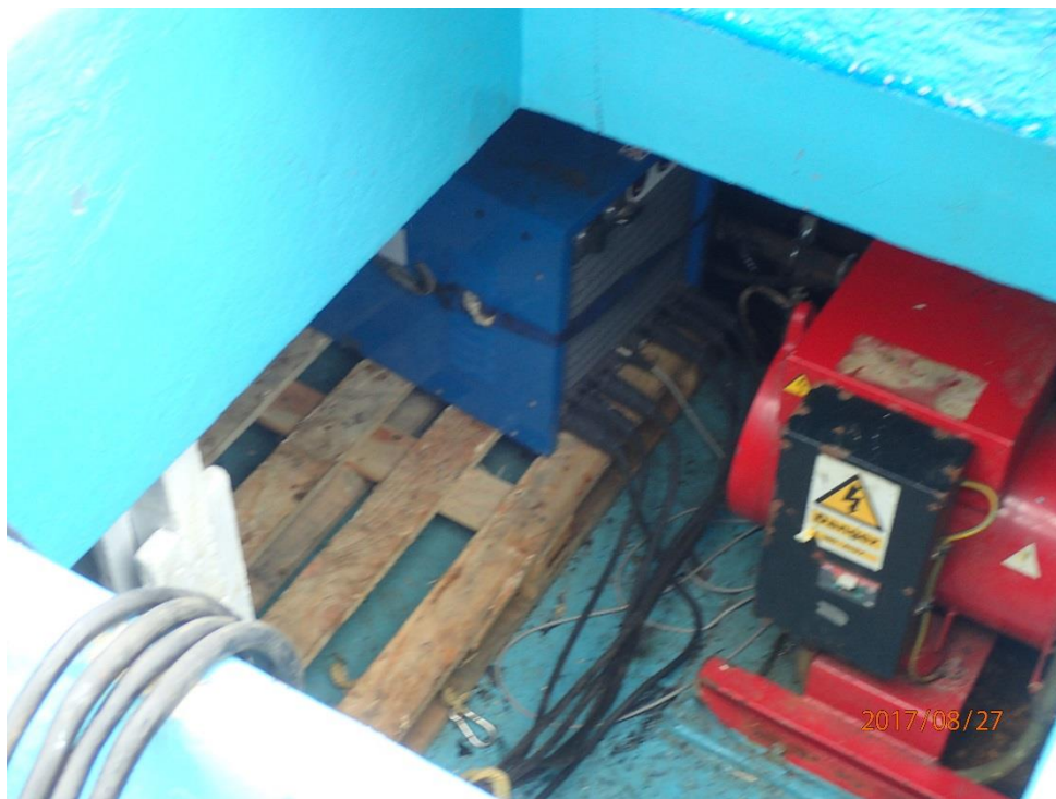
Figure 3: The blue inverter box sitting in the hold next to the generator (red painted equipment), the power outputs were monitored continuously in the bridge during fishing.
