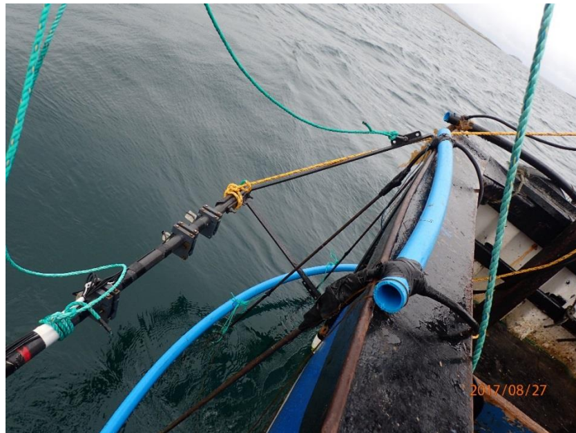
Figure 5: The video-rig being lowered off the back of the vessel, the blue bars are the electrode spreaders.
