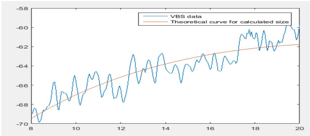
**Figure 10.** Volume backscattering spectrum (blue) from the upper middle section of the mackerel school in Fig.2 from the 424 channel and the fitted model (red) corresponding to a fish of length of 21.5 cm.
