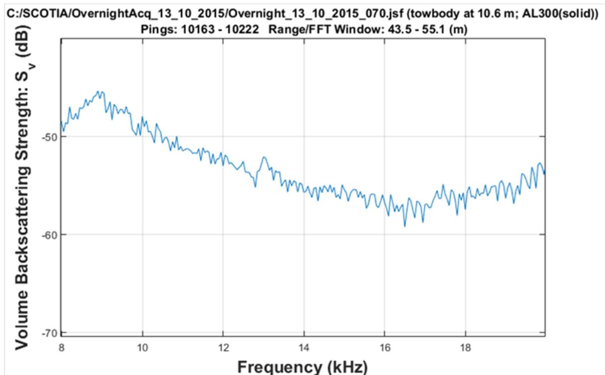
**Figure 8.** Volume backscattering spectrum from a school of myctophids using the 424 channel.
