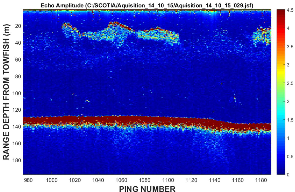
**Figure 2.** Echogram of a mackerel school from the EdgeTech broadband sonar. Depth on the y axis displayed as the range from the towfish (which was at a depth of 6 m). The ping number scale on the x axis, given a ping rate of 0.5 Hz and speed of 5 knots, equates to a total distance of approximately 1050 m. The colour scale is relative echo intensity: red is high, indicating strong echoes (fish schools and the seabed), blue is low (empty water).
