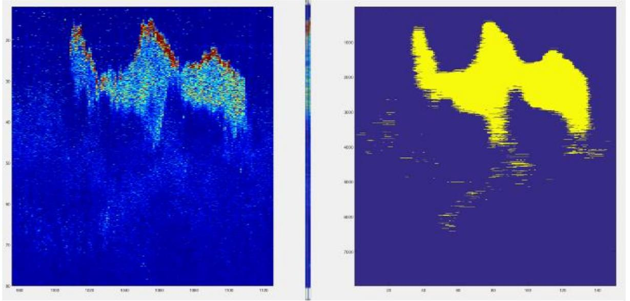
**Figure 5.** Echogram of a fish school (left) and the subsequent thresholded mask (right) used to isolate data from the fish school (only those points in yellow proceed to the image analysis for selection).
