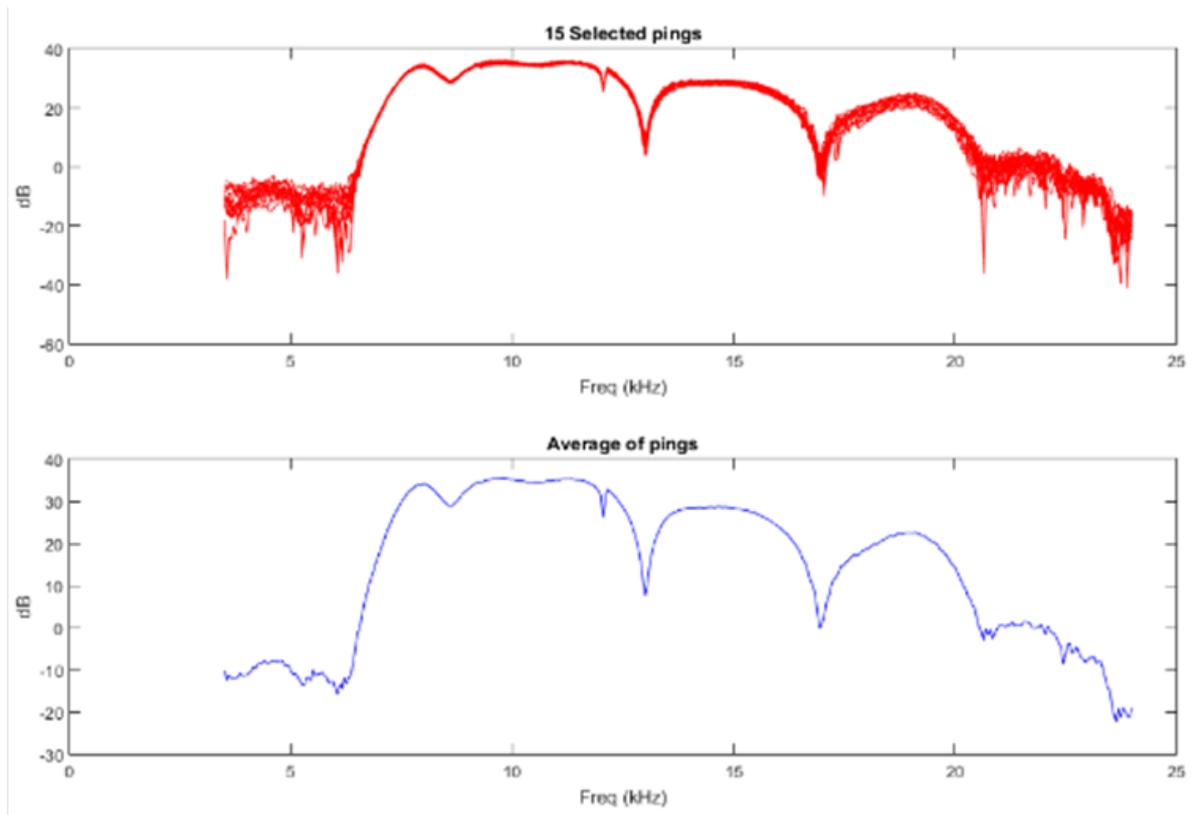
**Figure 4.** Volume backscattering spectrum of the calibration sphere from the 424 transducer. Top (red): Spectrum from 15 selected pings. Bottom (blue): average spectrum.
